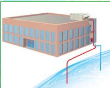
Open Loop Groundwater Well System
